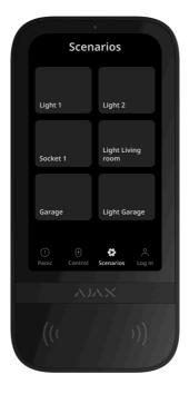
The separate keypad tab holds up to six buttons that control one <u>automation</u> device or a group of devices. Group scenarios provide more convenient control
