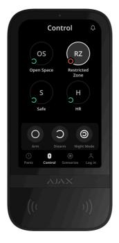
KeyPad TouchScreen allows controlling the groups' security (if **Group Mode** is enabled). You can also adjust the keypad **settings** to determine which groups will be shared (keypad groups). By default, all groups are visible on the keypad display in the **Control** • tab. You can learn more about group security management in **this section**.
