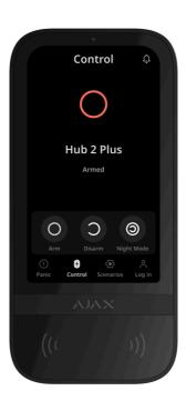
If Group Mode is enabled, users see the security mode of each group separately. The group is armed if its button outline is white and it is marked with  $\bigcirc$  icon. The group is disarmed if its button outline is grey and it is marked with  $\bigcirc$  icon.
