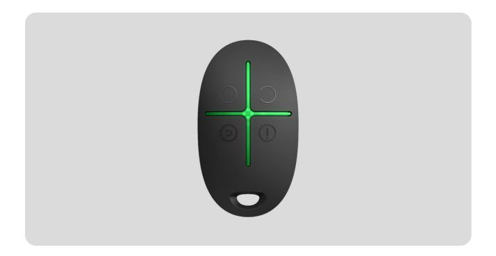
**Ajax SpaceControl** is a miniature key fob with accidental click protection. It allows setting the Ajax system in the armed, night or disarmed mode and switching on an alarm.
