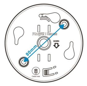
(2) Secure the mounting bracket to the ceiling or wall by using self-tapping screws.
