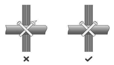
• When cables need to be bent, you should first bundle them up. However, the buckle cannot be bundled within the bend area. Otherwise, considerable stress may be generated in cables, breaking cable cores.
